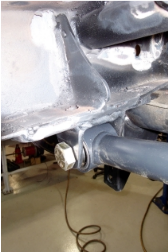
The panhard bar bracket is welded to the bottom of the rail and a gusset is welded into the inside of the rail to strengthen the area.
