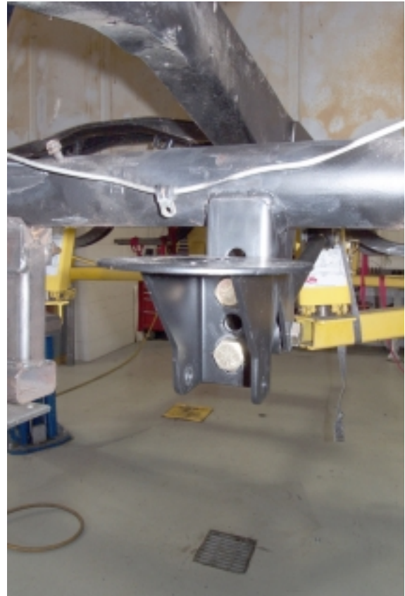
The lower air spring bracket bolts to the rear bar mount using the lowest holes.
