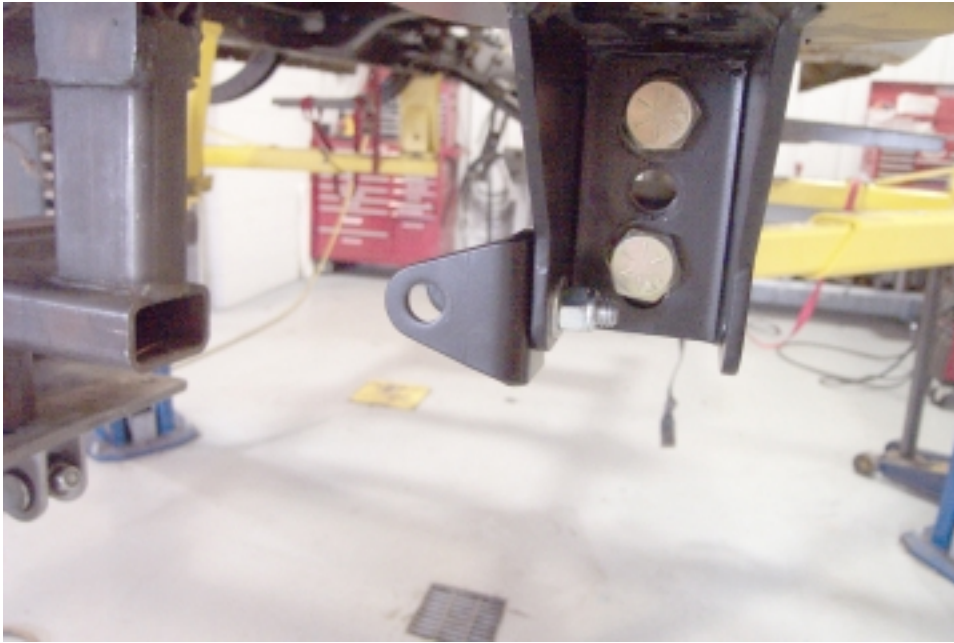
The lower shock mounts bolt to the inside of the lower spring mount.
