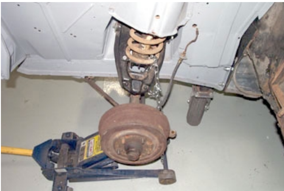
Jack stands to keep the car up and stable and a good floor jack make the work safer. Start by lifting the wheel up, but not enough to lift the car.
