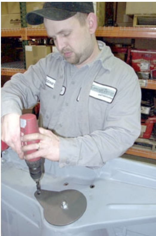
The top plate mount is formed so it will lie flat to the sheet metal with the center bolt at about the center of the tower opening. It only wants to fit one way. When positioned, Tighten the center bolt to hold it, and drill a 1/2 inch hole at the rear of the mount as shown here.
