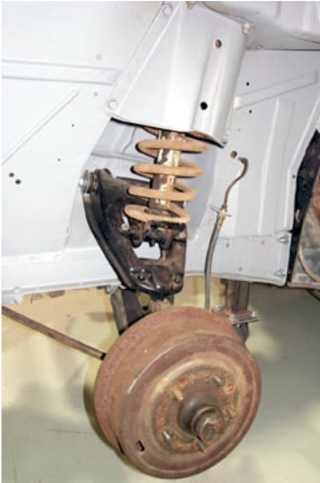
This is what you start with. The spring is positioned over a conventional triangulated upper A-arm while the lower arm uses a strut to stabilize it. There will be brake upgrades later, but for now it's worth seeing it go together nearly stock.
