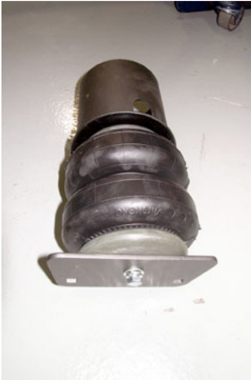
On the bottom, another bracket is bolted to the air spring. It's hard to get the bolt started after the mount plate is installed.
