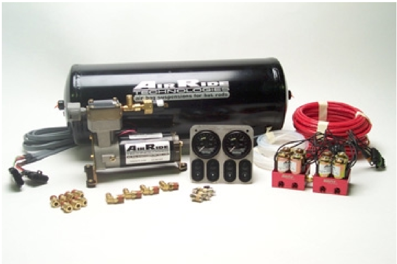
The high-end RidePro kit might contain pump, tank, lines and fittings, and then add digital gauges, solenoid-operated valving with micro-switches, and even a large-bore setup for rapid deployment called Big Red. Big Red uses 1/2 OD (3/8 ID) line and 3/8 ID valves for fast action.
