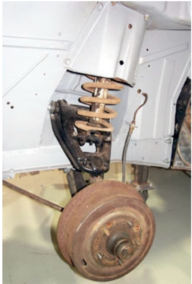
The original CII spring is positioned over a conventional triangulated upper A-arm while the lower arm uses a stabilizing strut. Like most upgrades, disc brakes will come later, but for now it's worth seeing it go together nearly stock.
