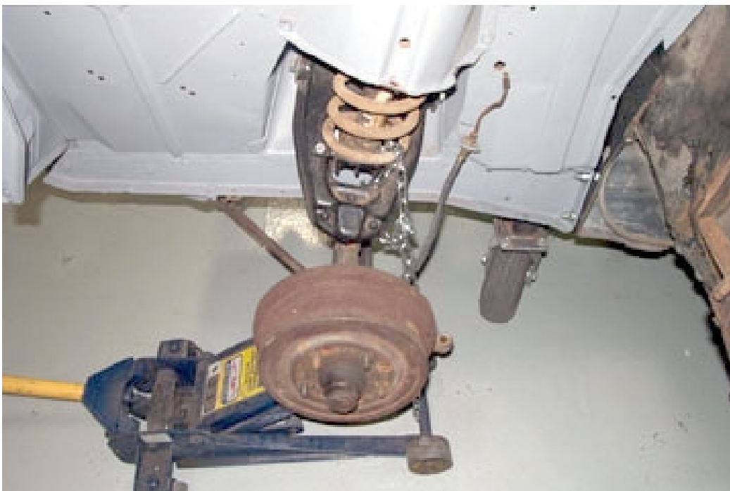
Always use jack stands to keep the car up and stable and a good floor jack make the work safer. Start by lifting the wheel up, but not enough to lift the car.
