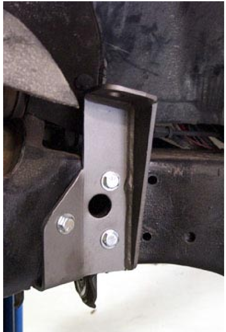
I like the way this bracket works because it requires no cutting or frame modification. Bolt the bracket to the side, mark and drill the bottom bolts, and install them to finish.
