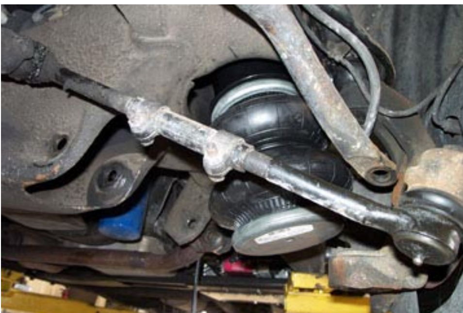
The assembly is slipped up into the spring tower and the stud up through the original upper shock mount. No cutting required.
