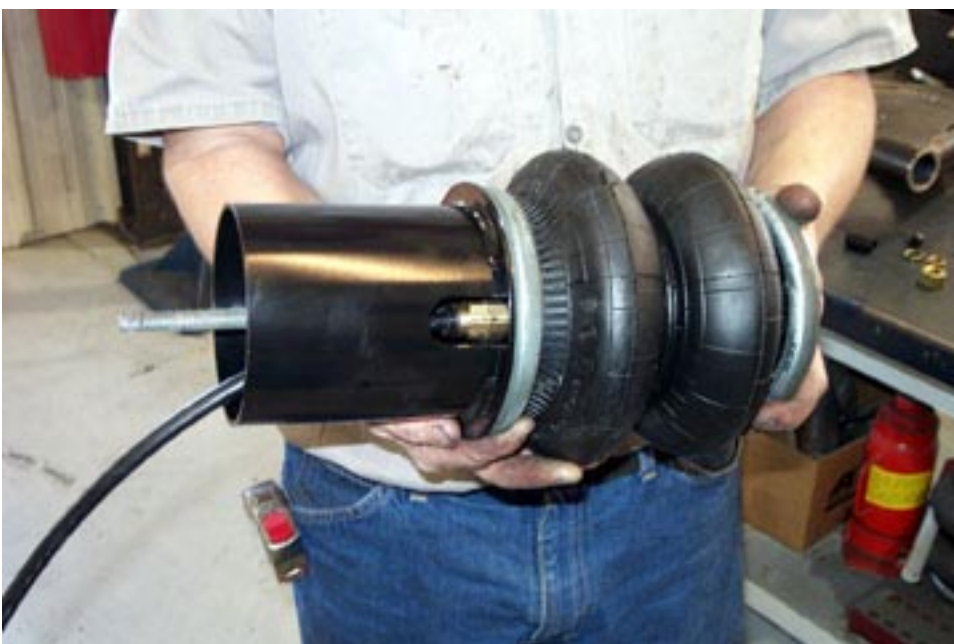
The air spring, air fitting, long stud, air line, and adapter are assembled as a unit.
