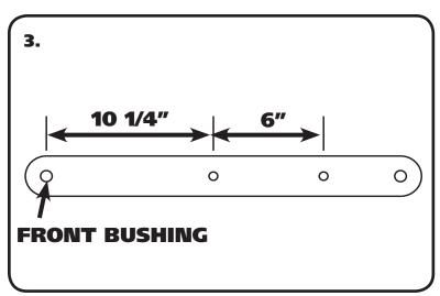
1. Holes will need to be drilled in the lower control arm to mount the rear swaybar. These holes should be drilled to 7/16". Measure back 10 1/4" from the center of the Front Bushing and make a mark centered top to bottom. Next measure back 6" from your first mark and Mark the Second Hole centered Top to Bottom. Drill the Locations with a 7/16" Drill Bit going through both Sides of the Arm. Repeat for both Arms.
