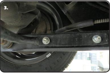
**3.** Slide the bar in Place with the CENTER OF THE BAR GOING UPWARD. Install a 7/16" washer on one of the 7/16"-14 x 3" Bolts and install one in each Front Hole to help hold it in place. Swing the SwayBar into position and insert the Rear Bolt/Washer. Tighten Hardware.
