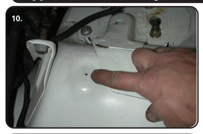
**10.** A bump stop will be installed between the inner fender and upper control arm to ensure that the tire does not hit the inner fender when fully compressed. There is a small hole on the inner fender that must be drilled out to 3/8". Fasten the bump stop to the inner fender using a 3/8" Nylok nut and flat washer.
