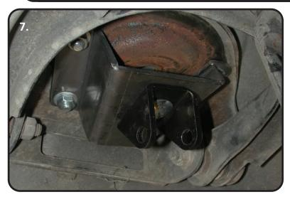
7. Using the 1/2" Carriage Bolt, 1/2" Flatwasher, and 1/2" Nylok, bolt the Upper Shock Mount to the upper bracket. The squares in the brackets should be aligned with the square shank on the carriage bolt. With the squares aligned tighten the mount. With the 2 pieces bolted together, bolt them into the car using (4) 3/8"-16 x 1 1/4", (8) 3/8" Flatwashers, and (4) 3/8" Nylok nuts. There is Driver and Passenger Bracket and this have a "D" and "P" stamped in them. Tighten all hardware.
