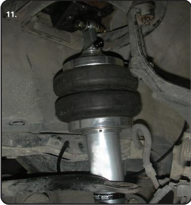
**11.** Route the Air line to the Valves. Be sure to stay away from heat sources and sharp edges.
