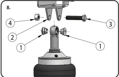
**8.** Thread the fitting into the ShockWave using Teflon tape on the threads. Assembly the spacers(1) into the bearing in the upper eyelet. With the spacers installed insert the ShockWave assembly into the upper shock mount(2). Align the holes in the bracket with the hole in the Shock spacers and insert the 1/2" Bolt(3) and secure with the 1/2" Nylok Nut(4).
