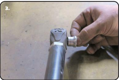
**3.** Press the SMALL diameter of the 9/16"I.D. R-Joint spacers into each side of the center ball of the remianing R-Joint. Push the spacers in until they bottom out in the center ball.
