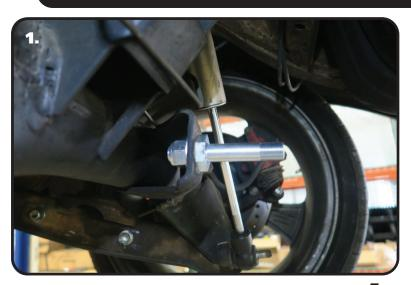
**1.** Bolt the new panhard bar stud into the OEM location of the axle using the 9/16" flat washer and 9/16"-18 Nylok nut supplied in the kit. Torque to 95 ftlbs.
