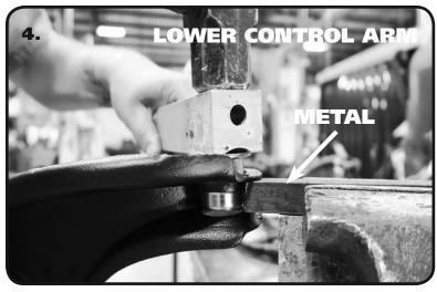
installed. If installing Bushings in the Upper Control Arm, insert the Cross Shaft before installing any Bushings. Support the Back Side of the Flange the Bushing is being Installed in. Use a STIFF piece of Metal clamped in a Bench Vise for the Lower Control Arms (Image 4). The Upper Control Arm can be supported by either the same piece of Metal or by the Bench Vise with the Jaws opened wide enough to let the Bushing Shell pass through (Image 5).
