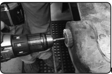
**3.** We recommend lightly sanding the bushing holes in the control arms to remove any debris that might be left in the holes after the bushings are removed. This will make the bushings easier to install.
