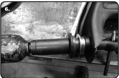
7. UPPER CONTROL ARM: (Image 6) Push the Inner Sleeve into the Delrin Bushing. Push the Delrin Bushing/Inner Sleeve assembly into the Outer Shells. They will go in partially. Install the OEM washer and nut on each end of the cross shaft. Tighten the Hardware on each end until the Delrin Bushings are bottomed out against the lip of the Outer Shell installed in the control arm.
