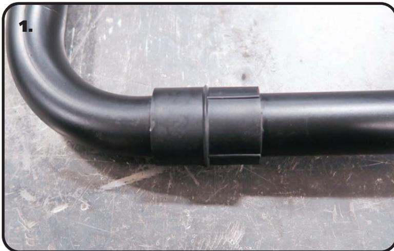
**1.** The Delrin Liner is split on one side to ease installation. We found it easier to install by opening up the Liner enough to slide it onto the end of the SwayBar, then sliding it into position. It will open up and slide over the curves in the Bar. Install a Liner on each side of the SwayBar in the approximate location they will need to be when installing the SwayBar on the Car.
