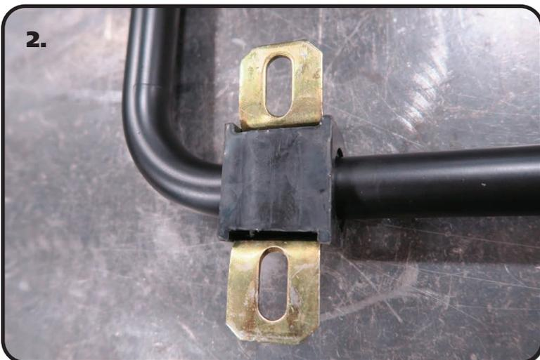
**2.** Open up the Poly SwayBar Bushings and install them over the Delrin Sleeves. Install Bushing Straps Over the Poly SwayBar Bushings.
