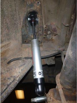
1. Unbolt the OEM shock and upper mount from the car.
