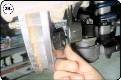
**23.** Insert the steering arm slugs into the spindle with the threads to the bottom of the spindle,
