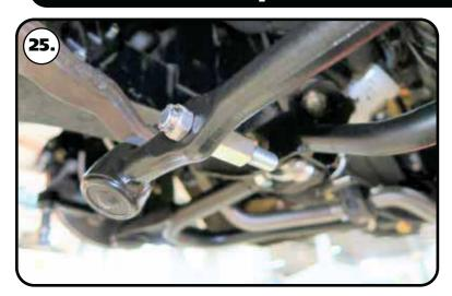
**25.** The studs with the long hex on them will get installed into the factory centerlink with the taper going into the centerlink, a 7/16" castle nut is used to attach it to the centerlink. The straight shank will point to the front of the car.
