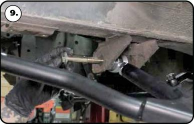
**9.** Align the factory holes with the control arm through hole. Install a 1/2" flat washer on a 1/2"-13 x 3 1/2" hex bolt. Insert the bolt/ washer through the aligned holes. Install a 1/2" flat washer and 1/2"-13 nylok nut on the threads of the bolt. Torque to 75 ftlbs.
