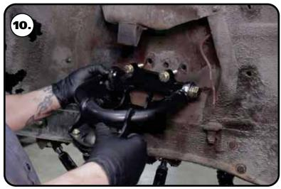
cars have been redrilled 1" lower. This is done to improve the handling. Our cross shaft has the drop built into it; make sure to use the factory mounting holes.
