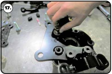
17. Insert a  $1/2"-13 \times 1 \ 1/4"$  flat head socket cap screw in each of the lower mounting holes. Install a 1/2" flat washer on a  $1/2"-13 \times 1 \ 1/4"$  hex bolt and insert it in the upper mounting hole. Tighten the hardware to 75 ft-lbs.
