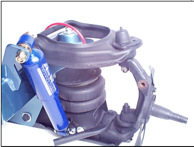
Mustang II with OEM lower a-arm
