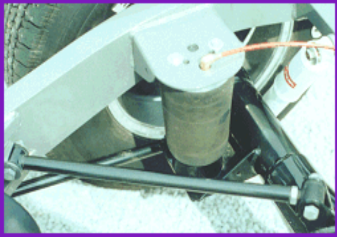
Rear suspension w/ 4 link and air ride
