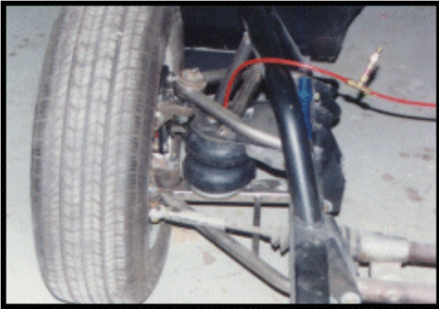
Aftermarket Mustang II installation [replaces coilover shock]
