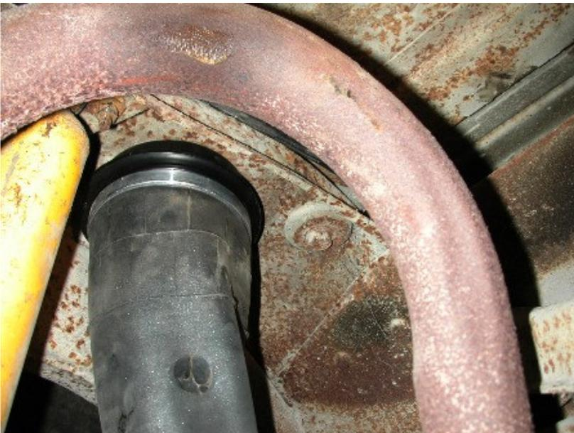
3. Apply thread sealant to a 90 deg. air fitting and screw it into the top of the air spring.
