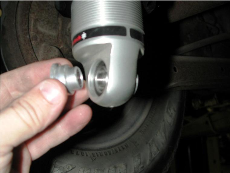
8. Install the aluminum spacers into the upper and lower eyes of the shock.
