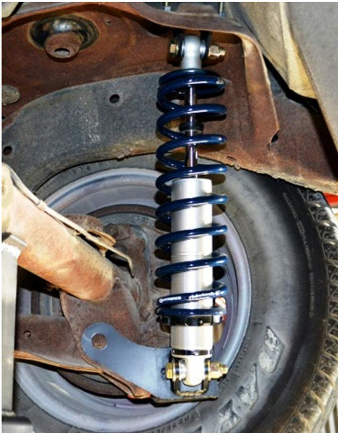
9. Fasten the shock to the upper bracket using a  $\frac{1}{2}$ " x  $2\frac{1}{2}$ " bolt and Nylok nut.
