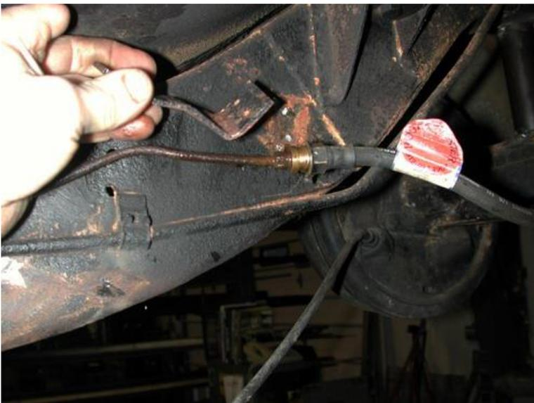
4. The rear brake line bracket on the passenger side fame rail must also be removed.
