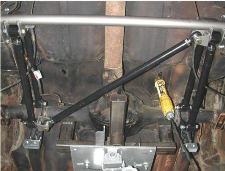
17. Bolt the lower Shockwave mount to the axle bracket using the 1/2"-20" x 3/4" Hex Head Bolt. Apply anti-seize to the threads. It is easier to remove the bars to install these bolts.
