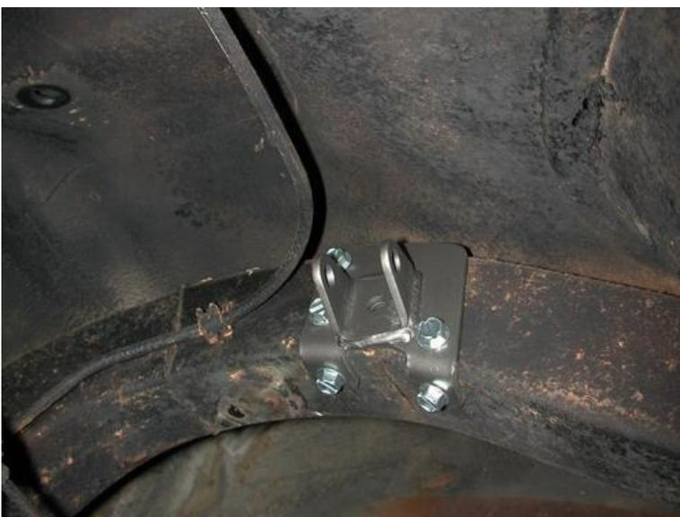
7. Use a clamp to hold the bracket against the inside of the frame and drill the holes with a 5/16" bit. Thread a 3/8" x 1" self-tapping bolt into the frame after drilling each hole.
