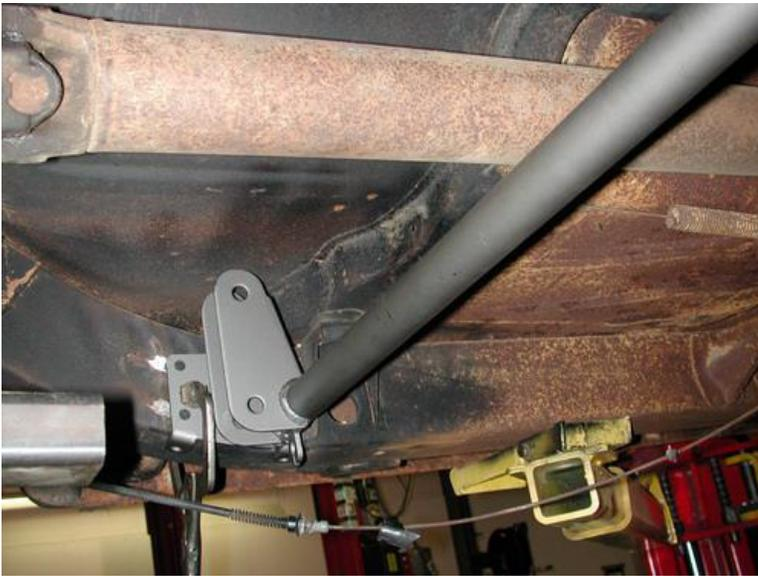
5. Use a couple clamps to secure the crossmember between the frame rails. Slide it forward to the edge of the body mounts. Drill the holes with a 5/16" bit and thread the 3/8" x 1" self-tapping bolts in one at a time.
