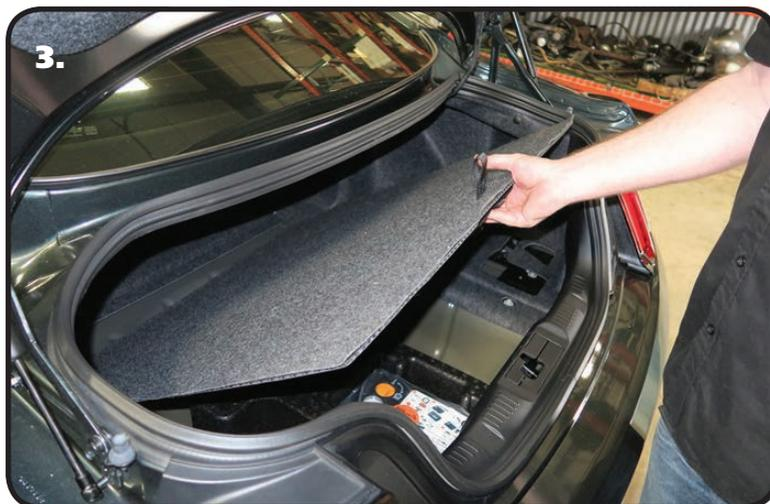
3. Start by removing the trunk floor cover exposing the spare tire well. This will make it easier to pull the passenger side trunk liner out of the way to access the module.
