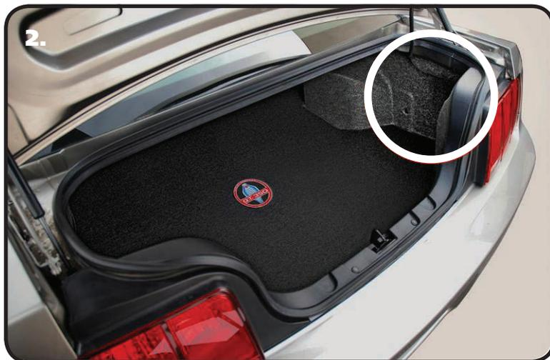
2. The OEM control module is located in the Passenger rear corner of the trunk behind the trunk liner.
