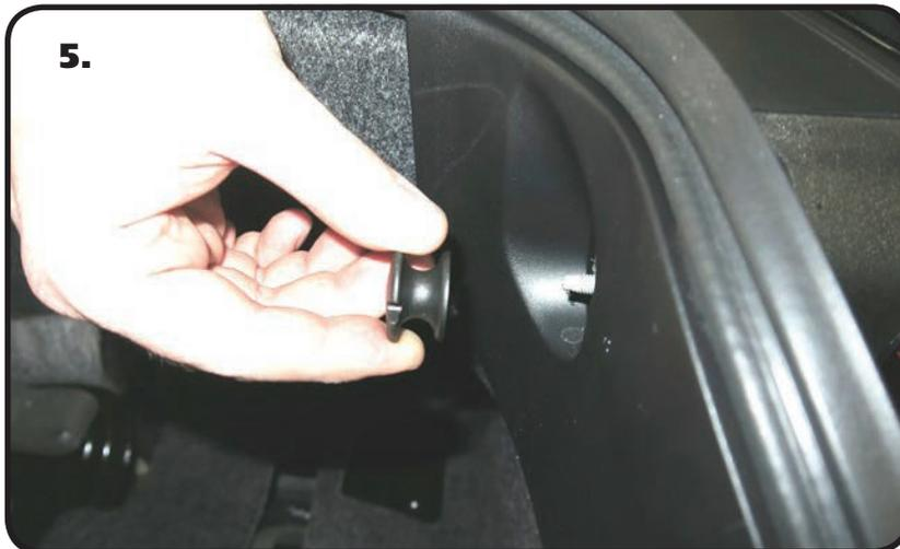
5. Remove the (2) rear panel retainers by threading them off. This will allow the corner of the panel to be pulled forward enough to pull the rear corner of the passenger liner out exposing the control module.
