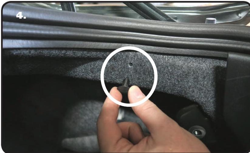
4. Remove the Black Retainer Plug out of the top of the passenger side trunk liner. This is located at the top of the liner, right below the trunk seal.
