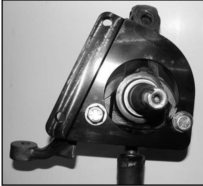
Figure 2: Rear Steer spindle shown with base bracket
