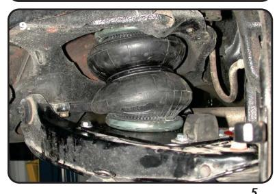
**9.** The air spring will be attached to the lower plate using a 3/8" x 3/4" bolt, lock washer and flat washer. It will get bolted to the middle of the 3 holes. Torque the 3/8" bolt 15-20 ft-lbs.
