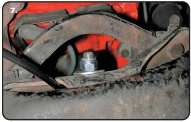
**7.** Fasten with a 7/16" Nylok nut and flat washer. Torque 25-35 ft-lbs.
