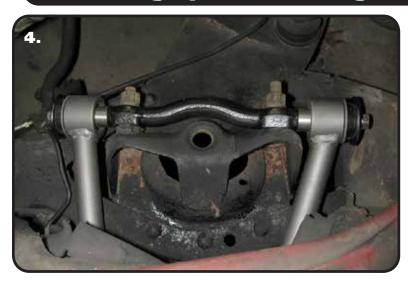
**4.** The Upper Control Arm is attaching the factory mount using factory hardware. Reinstall the shims in the location they were removed from. The passenger side arm is shown in **Figure "4"**. Torque the hardware 65-75 ft-lbs.
