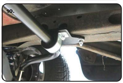
10. Install 3/8" Flat Washers on (2) 3/8" x 1 1/4" Hex bolts and install them through the top side of the of the remaining holes in each Mounting Plate with the threads pointing down. With the Delrin Liners/Bushings and Straps installed on the Sway Bar, put the swaybar in position on the 3/8" Bolts. Attach it using 3/8" Flat Washers and 3/8" Nylok Nuts. Do NOT completely tighten the Hardware. It will be left partially loose until the End Links are installed.
