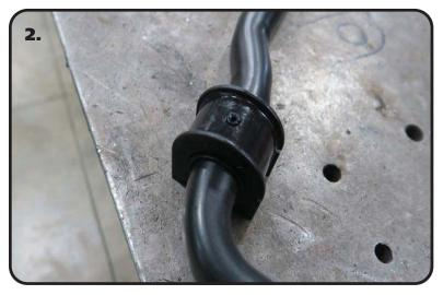
**2.** Open up the Poly Sway Bar Bushings and install them over the Delrin Sleeves.
