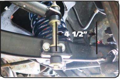
**4.** An End Link Mount will need to be added to the control arms, this requires drilling mounting holes in the control arm. The CENTER of the End Link Mount needs to be positioned 4 1/2" from the BACK edge of the ball Joint mounting bolt. The bottom of the mount will sit against the lip of the control arm. Use the End Link Mount as a template to drill the holes 3/8". Attach the mount using (2) 3/8" x 1" Hex Bolts, (4) 3/8" Flat Washers, & (2) 3/8" Nylok Nuts. Repeat on other control arm.
