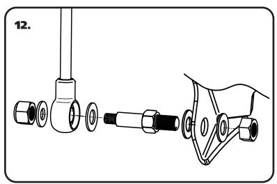
12. The Lower Shock is Bolted to the Lower Shock Mount using the supplied Shock Stud. Insert the Shock Stud into Lower Mount with a 5/8" Flat Washer on EACH side of the mount. Install a 5/8" Lock Nut on the threads and tighten. Next, slide a Washer on the Shock Stud. Jack the Rear Differential up until the Shocks can be slid onto the Shock Studs. Install a 7/16" Flat Washer and 7/16" Hex Nut onto the Threads and tighten.
