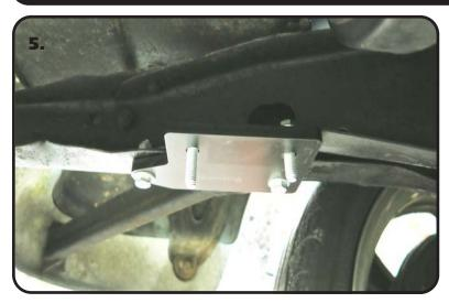
**5.** Install 3/8" flat washers on (2) 3/8" x 1 1/4" hex bolts. Install them through the top side of the of the remaining holes in each mounting plate with the threads pointing down. The rear bolt will also go through the frame rail.
