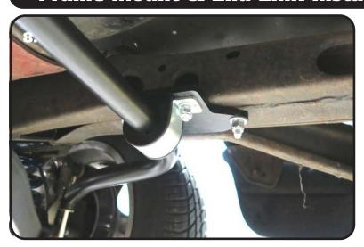
**8.** Install 3/8" flat washers on (2) 3/8" x 1 1/4" hex bolts and install them through the top side of the of the remaining holes in each mounting plate with the threads pointing down. With the bushings and straps installed on the sway bar, put the sway bar in position on the 3/8" bolts. Attach it using 3/8" flat washers and 3/8" nylok nuts. Do **NOT** completely tighten the hardware. It will be left partially loose until the PosiLinks are installed.
