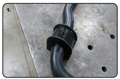
**1.** Apply lithium grease to the poly bushing. Install the bushing over the sway bar.
