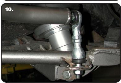
**10.** Bolt the straight end of the PosiLink to the lower control arm. An aluminum step washer must be installed on each side of the control arm tab. Fasten with a 10mm Nylok nut. Then tighten the bushing frame bolts.
