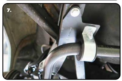
7. With the Delrin Liners/Bushings and Straps installed on the SwayBar, put the swaybar in position on the 3/8" Bolts. Attach it using 3/8" Flatwashers and 3/8" Nylok Nuts. Do **NOT** Complete tighten the Hardware. It will be left partially loose until the End Links are installed.
