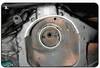
**3.** To allow clearance for the Shockwave, some trimming must be done on the outside edge of the coil spring pocket as shown by the white line in the picture. This is best done with either a cut off wheel or plasma cutter. Grind all cuts smooth when finished.
