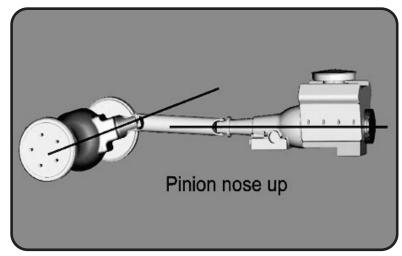
How do you set the pinion angle? On a singlepiece shaft you want to set it up where a line drawn through the center of the engine crankshaft or output shaft of the transmission and a line drawn through the center of the pinion are parallel to each other but not the same line.
