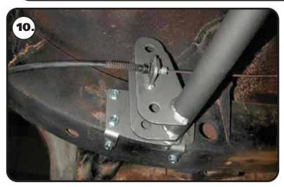
**10.** Reattach the emergency brake cables to the mounts built into the front cross member.
