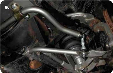
**9.** Bolt the 90 degree end of the PosiLink to the sway bar. A 3/8" flat washer and 10mm lock washer must be installed between the PosiLink and the bar.
