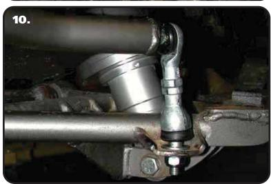
**10.** Bolt the straight end of the PosiLink to the lower control arm. An aluminum step washer must be installed on each side of the control arm tab. Fasten with a 10mm Nylok nut. Then tighten the bushing frame bolts.
