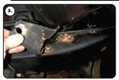
**3.** The parking brake brackets will be in the way of the 4 link and must be removed. Loosen the parking brake adjustment nut and remove the cable from the frame bracket. The tack weld can be broke loose with a hammer and chisel. Grind the remains of the weld smooth.
