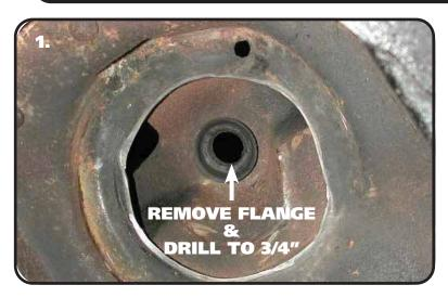
**1.** Remove the OEM bushing flange by prying it out of the frame hole. After removing the flange, drill the OEM shock hole out to 3/4". This can be done with a Unibit.
