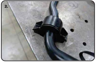
**2.** Install bushing straps over the poly sway bar bushings.
