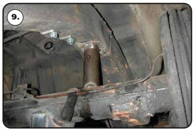
**9.** Pinion angle must be set at ride height. At ride height there should be 4 1/2" between the axle and frame. One trick to help maintain these setting while welding in the axle bracket is to tack weld a 4 1/2" long spacer between the axle and frame. **Refer to Page 8 for pinion angle setting.** After setting the pinion angle, make sure the axle is centered. This can done by measuring from the axle flange in to the frame rail.
