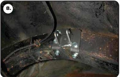
**8.** Use a clamp to hold the bracket against the inside of the frame and drill the holes with a 5/16" bit. Thread a 3/8" x 1" self-tapping bolt into the frame after drilling each hole.
