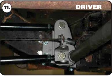
**11.** Insert the R-Joint spacers into the R-joint with the small OD inserted into the R-Joint center pivot. Install the 4 link bars into the crossmember. Use the 5/8" x 2 3/4" bolts and nyloks supplied in the mounting holes that don't have a diagonal bar mount. The holes that have a diagonal link bar mount use a 5/8" x 3" bolt and nylok. Tighten the bolts/nuts enough to eliminate any gaps.
