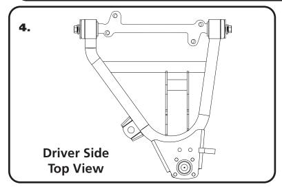
**4.** The Lower Control Arm is attaching the frame using factory hardware. The driver side arm is shown in **Figure "2"**. The sway bar mount is located to the front of the car.
