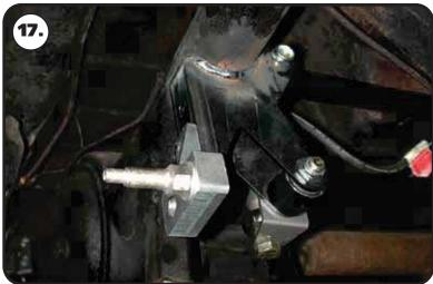
17. Installing the shock stud into the outer hole of the lower mount. Install a 5/8" flat washer onto the 5/8"-18 threads of the shock stud. Apply Red Loctite to the 5/8" threads of the stud. Thread the shock stud into the threaded hole of the lower mount. Repeat on both sides and torque the shock stud to 65-75 ft-lbs.
