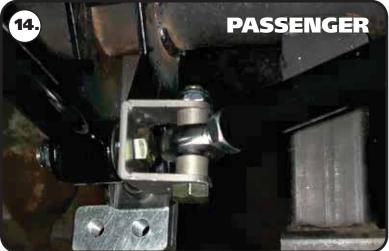
**14.** Insert the R-Joint spacers into the R-joint with the small OD inserted into the R-Joint center pivot. Bolt the diagonal link into the mount on the passenger axle mount using a 5/8" x 2 3/4" bolt and nylok. Tighten the bolts/ nuts enough to eliminate any gaps.
