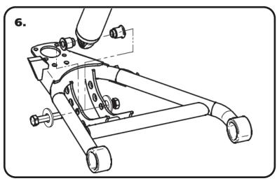
**6.** Bolt the Shockwave or CoilOver to the lower arm using the supplied 1/2" x 3 1/2" bolt, 1/2" flat washers, and 1/2" nylok nut. Insert the supplied aluminum spacers in each side of the shock bearing and slip it into the control arm. Line the spacers/bearing up with the 1/2" hole in the shock straps of the control arm and install hardware. Torque the hardware to 75 ftlbs.
