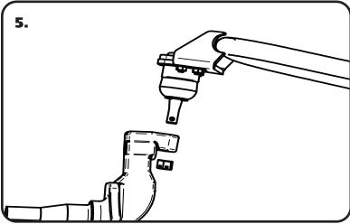
**5.** Attach the Spindle to the control arms. These control arms use a tall ball joint, the boot will NOT touch the spindle. This is normal.
