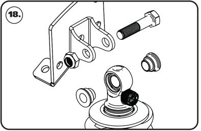
**18.** Install a 1/2" ID 90002043 spacer on each side of the upper Coilover/ShockWave. Slide the assembly into the upper crossmember from the bottom side. Position the adjuster knob so that the knob points toward the center of the car. Line up the hole in the spacers with the hole in the upper shock bridge and insert 1/2"-13 x 2 1/4" bolt and install 1/2"-13 thin nylok nut. Torque to 21 ft-lbs.
