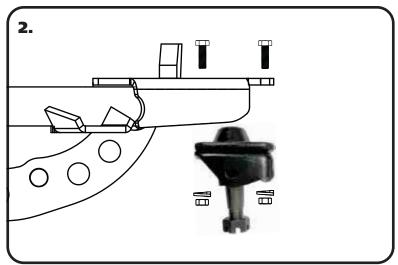
2. Insert the Ball Joint into the Control Arm from the bottom side with the Stud pointing downward. Insert the supplied Bolts from the top side. Install a Lock Washer and Hex Nut on the threads of each bolt. Torque the hardware to 25 ftlbs.
