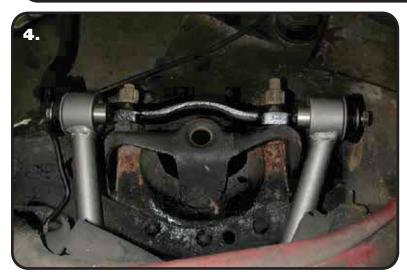
**4.** The Upper Control Arm is attaching the factory mount using factory hardware. Reinstall the shims in the location they were removed from. The passenger side arm is shown in **Figure "4"**.
