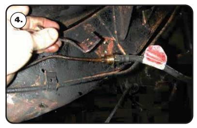
**4.** The rear brake line bracket on the passenger side fame rail must also be removed.
