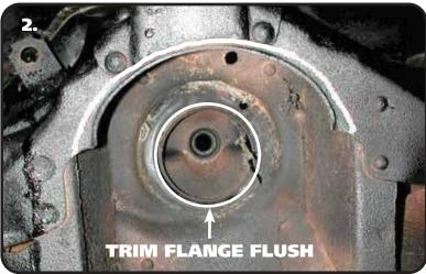
**2.** Trim the coil spring location ring flush to prevent the ring from hitting the top of the ShockWave Air Spring. A die grinder with a cutoff wheels works well here.
