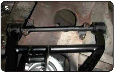
**5.** The Lower Control Arm is attaching the frame using factory hardware. The driver side arm is shown in **Figure "3"**.
