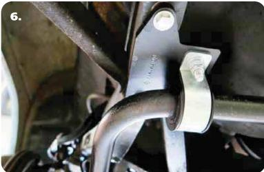
**6.** With the bushings and straps installed on the sway bar, put the swaybar in position on the 3/8" bolts. Attach it using 3/8" flat washers and 3/8" nylok nuts. Do **NOT** completely tighten the hardware. It will be left partially loose until the PosiLinks are installed.
