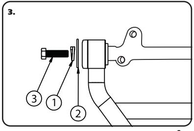
**3.** Install the supplied 7/16" Lock Washers & 7/16" Flat Washers on each of the (4) 7/16"-20 x 1 1/2" Bolts supplied in the kit. Thread each Bolt/Washer setup into the end of the Cross Shaft of the Lower Control Arm. Do not tighten until the control arms are installed on the car.
