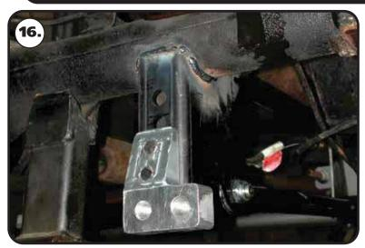
**16.** Bolt the lower Shockwave mount to the axle bracket using (2) ½"-20" x 3/4" hex head bolts. The mount offsets the lower shock stud to the outside of the car. Attach the mount to the **2 BOTTOM** holes of the axle mount. Torque the bolts to 75 ft-lbs.
