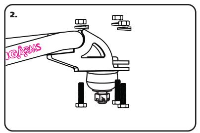
2. Insert the Ball Joint into the Control Arm from the TOP side with the Stud pointing downward. Insert the supplied Bolts from the bottom side. Install a Lock Washer and Hex Nut on the threads of each bolt. Torque the hardware to 18 ftlbs.
