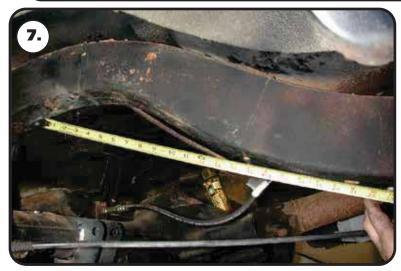
**7.** The location of the upper Shockwave mount is determined by measuring from the front edge of the bracket to rear edge of the large hole in the bottom of the frame. The location of the large locating hole varies between the 1 piece frame and 2 piece frame. Use the correct measurment from below to locate your shock mount.
