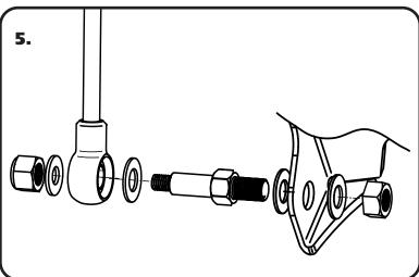
**Composite Leaf Spring Note:** When tightening the mounts, pay attention to the pads on the springs to make sure there is visible compression of the pads. .030"- .060" of compression is needed for the springs to be securely mounted. All of the clamping force needs to be on the spring itself.
