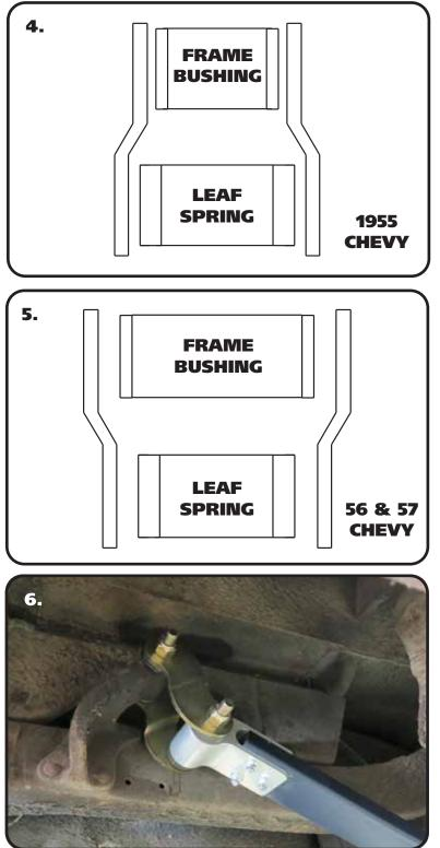
**4.** The orientation of the Shackle Plates is determined by the year of the car. The Frame bushing is 2 1/2" wide on a 1955, 3 1/2" wide on 1956-1957. 1955 is shown in Diagram "6". The 1955 uses 1/2"-13 x 4" in the FRAME bushing and 1/2"-13 x 4 1/2" in the REAR leaf spring bushing.
