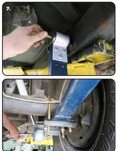
**7.** Bolt the **NARROW BUSHING END** of the Composite Leaf Spring into the OEM front leaf spring mount using a 1/2"-13 x 4" Hex Bolt and 1/2"-13 Nylok Nut.
