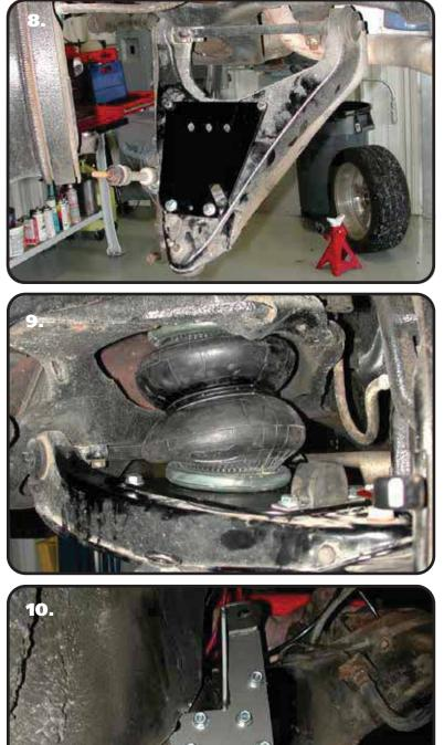
**8.** Bolt the lower air spring plate to the lower arm. The two outer holes will align with the factory bump stop holes. The inner two holes must be drilled. Use the bumpstop to bolt the outer part of the plate to the control arm. Use a 3/8" drill bit to drill the inner 2 holes. Instal a 3/8" flat washer on each of (2) 3/8"-16 bolts and insert them into the holes. Install a 3/8" flat washer and 3/8"-16 nylok nut on the threads of the bolt. Torque to 30 ft-lbs.
