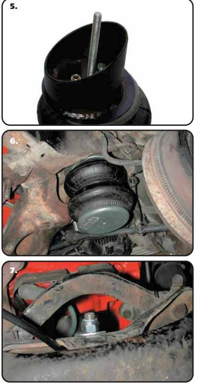
**5.** Thread the 8" stud into the nut in the bottom of the cup.
