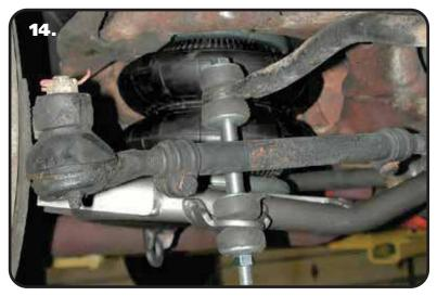
**14.** To correct the sway bar alignment the end link must be shorten to 2'' tall. A  $3/8''-16 \times 6$   $\frac{1}{2}''$  bolt is supplied.
