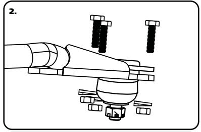
2. Insert the Ball Joint into the Control Arm from the TOP side with the Stud pointing downward. Insert the supplied Bolts from the top side. Install a Lock Washer and Hex Nut on the threads of each bolt. Torque the hardware to 18 ftlbs.
