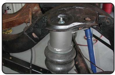
**3.** Apply thread sealant to the air fitting and screw it into the air spring. Assemble the upper cup bracket to the air spring, using 3/8"-16 Nylok nuts and 3/8" flat washers. Torque the 3/8" nuts 15-20 ft-lbs.
