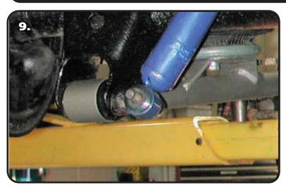
**9.** Attach the bottom of the shock to factory shock stud using the  $\frac{1}{2}$ " Nylok nut & flat washer supplied. Torque to 45 ft-lbs.
