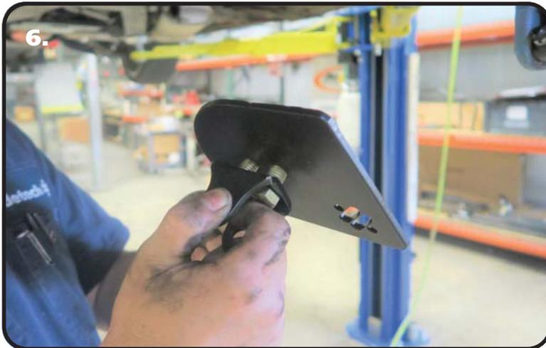
**6.** The Upper Mount is attached to the frame using (2) 1/2"-13 x 1 1/2" Bolts. Insert the bolts through the shock mount and into the upper plate.
