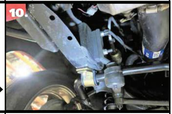
**10.** Reattach the idler arm to the frame using the OEM hardware. Torque the hardware.
