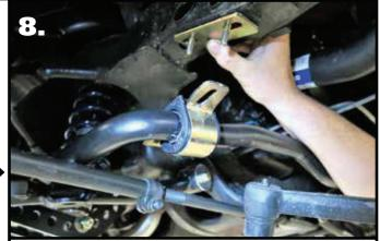
**8.** Install the bushing strap over the swaybar bushing with the wide side of the strap to the inside on the car. We found some steering box coversions hang down further than others. If yours happens to hit the sway bar, add a 2nd spacer under the bushing. a 2nd set of spacers along with longer hardware is supplied in this kit.
