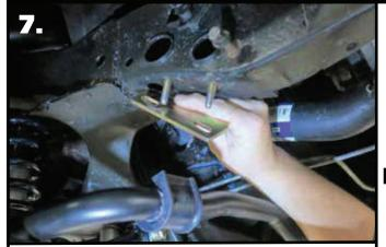
**7.** Install a 5/16" flat washer on each of (2)  $5/16"-18 \times 1 1/4"$  bolts and insert them into the OEM sway bar holes by inserting them in through the access holes in the side of the frame. Install the spacer plate with the wide side positioned to the inside. Hold it in place.
