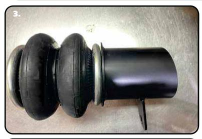
**3.** Apply thread sealant to the air fitting and screw it into the air spring. Assemble the upper cup bracket to the air spring, using 3/8"-16 Nylok nuts and 3/8" flat washers. Torque the 3/8" nuts 15-20 ft-lbs.
