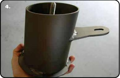
**4.** Thread the 6" stud into the nut in the bottom of the cup.
