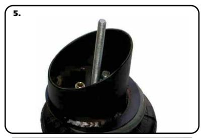
**5.** Thread the 8" stud into the nut in the bottom of the cup.
