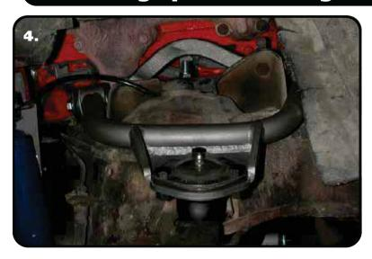
**4.** The Upper Control Arm is attaching the factory mount using factory hardware. Reinstall the shims in the location they were removed from. The passenger side arm is shown in **Figure "4"**. Torque the OEM nuts to 50 ft-lbs.
