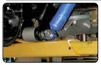
**9.** Attach the bottom of the shock to factory shock stud using the ½" Nylok nut & flat washer supplied. Torque to 45 ft-lbs.
