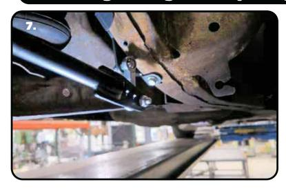
7. Install the PosiLinks in the frame brackets and in the FRONT hole in the MuscleBar. The Posilinks are installed with the stud on the upper PosiLink pointing outward and the stud on the lower Posilink pointing to the inside of the car. Install the 10mm Nylok on Posilink and tighten nut.
