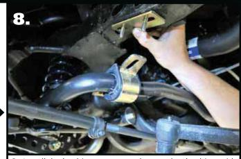
**8.** Install the bushing strap over the swaybar bushing with the wide side of the strap to the inside on the car. We found some steering box coversions hang down further than others. If yours happens to hit the sway bar, add a 2nd spacer under the bushing. a 2nd set of spacers along with longer hardware is supplied in this kit.
