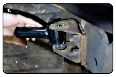
1. Insert the Bushing end of the Upper Control Arm into the OEM mount. The control arm should be installed with the bend upward for better axle clearance. Install a 5/8" flat washer on a 5/8"-18 x 3 3/4" hex bolt through the mount and control arm bushing. Install a 5/8" flat washer, followed by a 5/8"-18 nylok jam nut onto the threads of the bolt. Tighten the hardware enough to eliminate any gaps.
