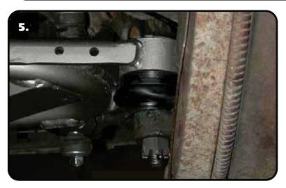
**5.** Attach the Spindle to the control arms. These control arms use a tall ball joint, the boot will NOT touch the spindle. This is normal.
