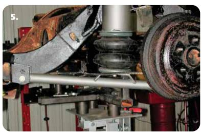
**5.** Fasten the air spring to the lower StrongArm using a 3/8" x 3/4" bolt, lock washer and flat washer. Torque 15-20 ft-lbs.
