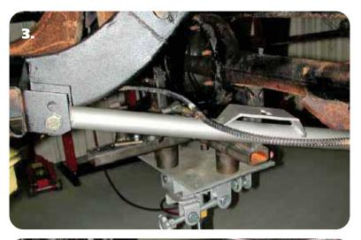
**3.** Fasten the front of the lower StrongArms to the frame using the 5/8" x 3 ¾" bolts, flat washers, and nylok nuts supplied. The OEM rear bolt will be reused in conjunction with the supplied flat washer and Nylok nut. Tighten the bolts/nuts enough to eliminate any gaps.
