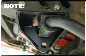
**NOTE:** IF YOUR CAR HAS THE FACTORY POWER STEERING SLAVE CYLINDER, KIT 11059121 WILL BE NEEDED TO INSTALL THE STREETGRIP SWAYBAR
