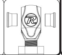
New R-Joints will be quite stiff (75-90 in/lbs breakaway torque) until they "break in" after a few miles of use. After the break in period they will move much more freely. Because the composite bearing race contains self lubricating ingredients, no additional lubrication is needed or desired. Any additional lubrication will only serve to attract more dirt and debris to the R-Joint and actually shorten its life.
