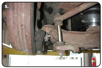
**5.** For better sway bar alignment the end link must be cut down by 1" to 2  $\frac{1}{2}$ " long. 3/8" x 6 1/2" Hex Bolts and 3/8" Nylok Nuts are included in the kit to replace the OEM hardware after shortening the sway bar end link.
