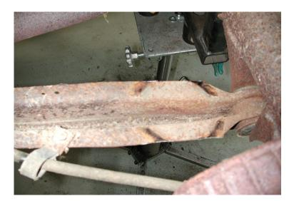
3. The lower coil spring retainer must be removed by cutting the welds. Grind all sharp edges smooth.
