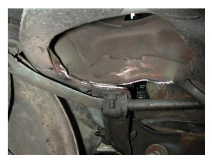
4. After double checking Shockwave clearance grind all edges smooth and paint exposed metal.
