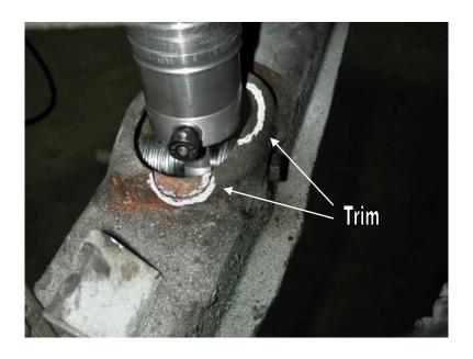
5. The lower control arm must be clearance as well to allow clearance for the shock body and the adjustment knob.
