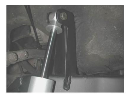
8. Place the air spring assembly into the coil spring pocket with the stud sticking through the "L" bracket. The assembly should be clocked so the air fitting faces the spindle. Secure with a 7/16" Nyloc nut and flat washer.
