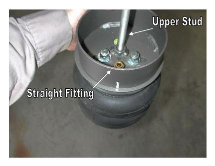
6. Thread the 6 ½" stud into the nut in the bottom of the bracket.
