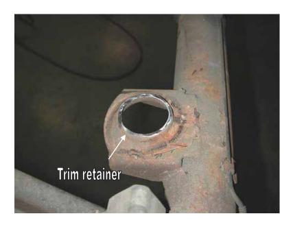
3. To allow the lower piston of the air spring to seat down into the coil spring retainer, the top of the retainer must be trimmed off.
