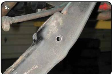
**5.** The lower shock mount hole will be used to mount the Shockwave. This hole must be drilled out to ½".
