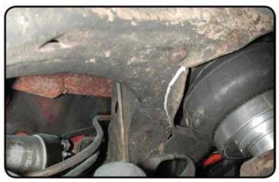
**4.** To allow for proper Shockwave clearance, so trimming must be done the lip around the coil spring pocket. This can be done with a die grinder and cut off wheel.
