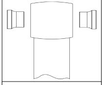
Insert the SMALL end of the spacer INTO each side of the center pivot ball. Push the spacer in until it bottoms out in the center pivot.
