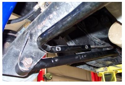
4. Attach to rear of the lower StrongArm to the frame using the ½" x 3 ½" bolts and Nylok nuts supplied.
