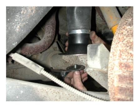
6. Hold the air spring assembly up to the coil spring pocket with the stud protruding through the hole in the center of the coil spring pocket. Place the 4" diameter washer over the stud and tighten with a 7/16" Nyloc nut and flat washer.
