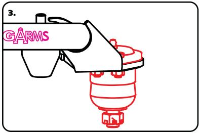
**3.** Install the Ball Joints in the control arms using **Figure "3"** as a reference. Torque the hardware to 15 ftlbs
