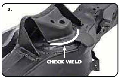
**2.** Check the weld in the area pointed out. We have seen some very poor factory welds in this area. If it doesn't look adequate to support the vehicle, reweld the area.
