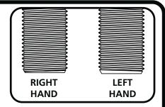
THE 4-LINK BARS, R-JOINTS, AND JAM NUTS HAVE RIGHT HAND AND LEFT HAND THREADS. THIS ALLOWS THE BAR TO BE ADJUSTED WITHOUT REMOVING IT. THE HEX END OF THE BAR IS LEFT HAND THREAD. THE LEFT HAND JAM NUT HAS AN COUNTER-CLOCKWISE ARROW STAMPED INTO IT. IMAGE 3 WILL HELP YOU DETERMINE THE THREADS OF THE R-JOINTS.
