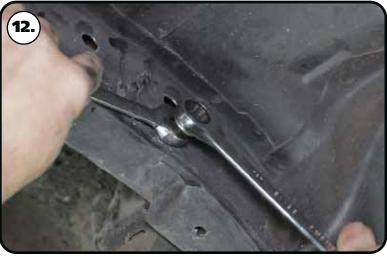
12. Install the Riv-nuts in the frame rails. Refer to the Riv-nut installation instructions on PAGE 8 for proper Riv-nut installation. Image 12 illustrates a Riv-nut being installed. Install all (18) Riv-nuts in the frame rails.
