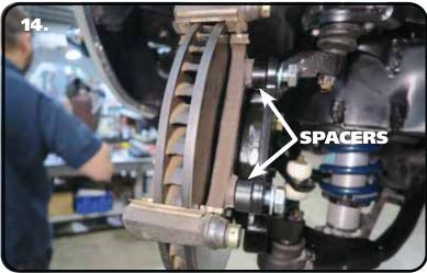
**14.** The kit includes spacers that will be installed between the caliper bracket and caliper mount. Install a M14 flat washer on each of (2) M14-2.0 x 45mm hex bolts. Insert the bolts through the caliper bracket, installing a spacer on each bolt. Line the caliper mount up with the hardware and thread in the bolts.
