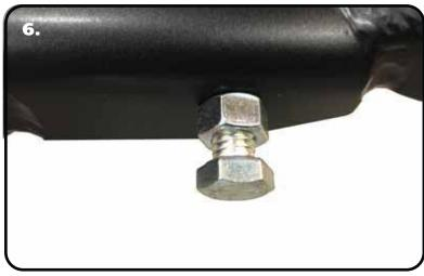
**6.** Thread the 3/8"-16 nut onto the 3/8"-16 x 1 ¼" bolt. Thread it into the front hole of the ball joint plate. You will need to adjust the steering stop to suite your needs. This setting will vary depending on wheel and tire size and other suspension components. Torque to 12 ft-lbs.
