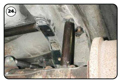
**24.** One helpful trick to help maintain ride height and pinion angle while adjusting is to tack weld a spacer between the axle and the outside of the frame as shown in the picture. This spacer should be 8 1/2" tall giving the Shockwave an eye-to-eye measurement of approximately 14 1/2". When measuring the axle center you can measure off of the frame rails. We also use a plum bob off the quarter panels to double check the axle center. Refer to **Page 14** on setting the pinion angle.
