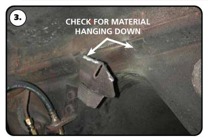
**3.** Remove the factory pinion snubber and mount from the car, this is necessary for clearance of the upper cradle. We use a cut off wheel to remove the mount. Make sure the area where the ARROW is pointing has no material sticking down. The tabs that are against the body can remain. Check both sides where the snubber mount attached to the body.
