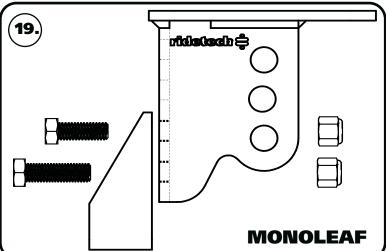
19. MONOLEAF - The Monoleaf setup uses the BOTTOM 2 HOLES for mounting. Insert the bolts through the aluminum shock mount with the 1 1/4" long bolt in the top bolt, 1 3/4" in the bottom hole. Insert the bolts through the axle mount and install the nylok nuts on the threads sticking through. Repeat on both sides and torque the bolts/nuts to 75 ftlbs.
