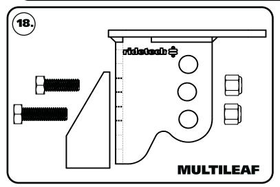
**18. MULTILEAF -** The Multileaf setup uses the **MIDDLE 2 HOLES** for mounting. Insert the bolts through the aluminum shock mount with the 1 1/4" long bolt in the top bolt, 1 3/4" in the bottom hole. Insert the bolts through the axle mount and install the nylok nuts on the threads sticking through. Repeat on both sides and torque the bolts/nuts to 75 ftlbs. Skip to **Step 20**.
