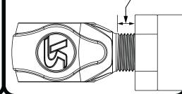
New R-Joints will be quite stiff (75-90 in/lbs breakaway torque) until they "break in" after a few miles of use. After the break in period they will move much more freely. Because the composite bearing race contains self lubricating ingredients, no additional lubrication is needed or desired. Any additional lubrication will only serve to attract more dirt and debris to the R-Joint and actually shorten its life.
