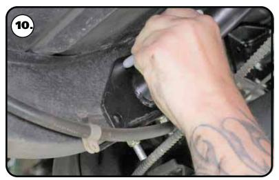
**10.** Mark the holes of the frame mounts. Mark the slotted holes in the center of the slot. These holes use Riv-nuts to bolt the cradle to the frame. The holes need to be centered as much as possible. Make sure to mark all (9) holes in each frame rail.
