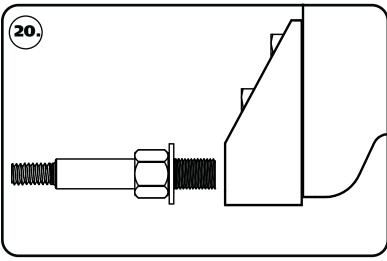
**20.** Installing the shock stud into the lower mount. Install a 5/8" flat washer onto the 5/8"-18 threads of the shock stud. Apply Red Loctite to the 5/8" threads of the stud. Thread the shock stud into the threaded hole of the lower mount. Repeat on both sides and torque the shock stud to 65-75 ftlbs.
