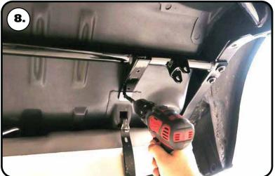
**8.** Drill a 3/8" hole through the each of the sway bar mount tabs. These holes will go into the trunk so make sure nothing is in the trunk floor. If there is a mat, remove it before drilling the holes.
