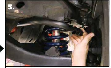
**5.** Insert the sway bar in the stock location. See below for installation tips.
