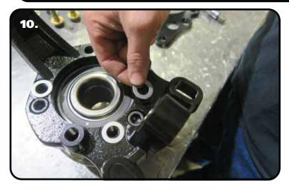
**10.** Lay a .062" thick, 1/2" ID shim on each of the caliper brackets (3) mounting holes.
