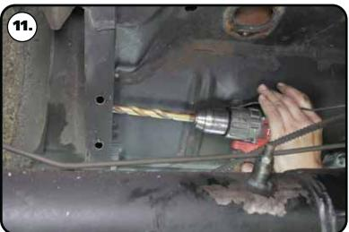
11. Remove the cradle to drill the holes and install the Riv-nuts. The holes for the Riv-nuts NEED to be drilled with the supplied 17/32" drill bit. We suggest drilling the holes with a smaller drill bit first to make it easier to drill with the 17/32" drill bit. Drill all (18) holes in the frame rails.
