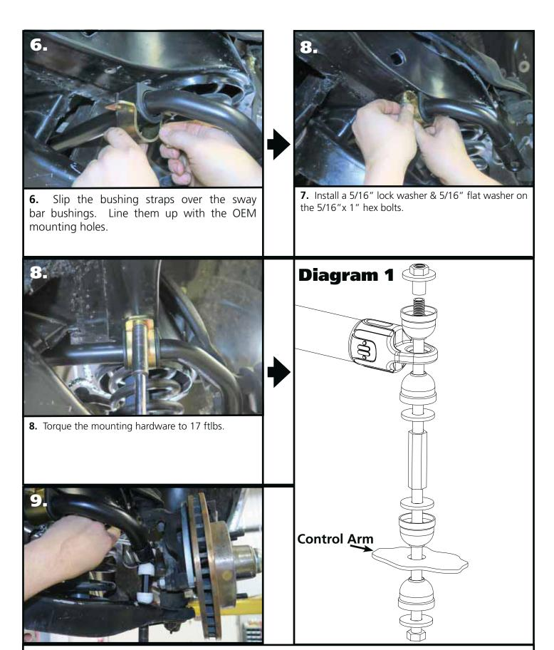
**9.** Install the end links using **Diagram 1** as a reference. Install both end links before tightening the end link hardware. Tighten the end link barrel nut until it is flush with the end of the bolt, and then tighten it 2 more complete rounds.
