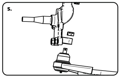
**5.** Attach the Spindle to the control arms.
