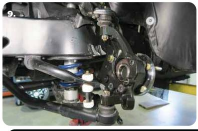
**9.** Attach the spindles to the control arms. Torque the ball joints using the torque specs below.
