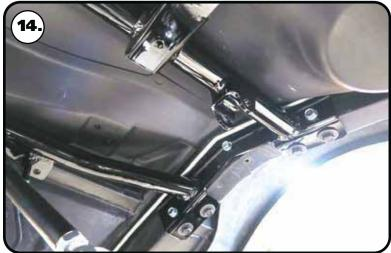
**14.** Install a 3/8" split lock washer & 3/8" flat washer on each of the 3/8"-16 x 1 1/4" bolts supplied in the kit. Thread them into the rivnuts. Torque to 23 ft-lbs. Torque the front tab and sway bar tab hardware to 30 ft-lbs.
