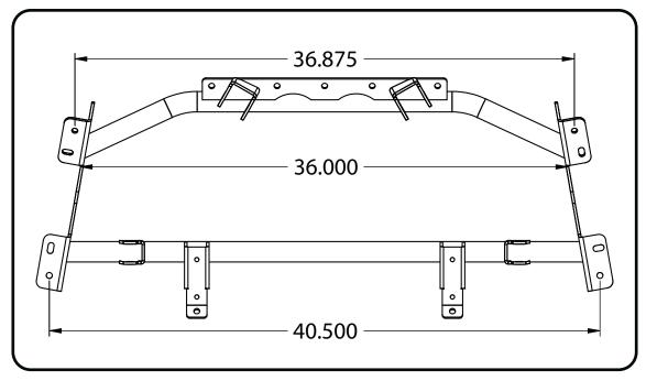
**Note**: In rare cases, the dimension from frame rail to frame rail on your F-Body may vary from the dimension on the Ridetech Upper Cradle. **ALL** of the Ridetech Upper Cradles are jig built to the dimensions above. The variation in OEM manufacturing specs does happen and is out of our control. If your F-Body frame rails seem out of spec, feel free to contact our Tech Department at 812-482-2932 and we will try to offer some solutions.
