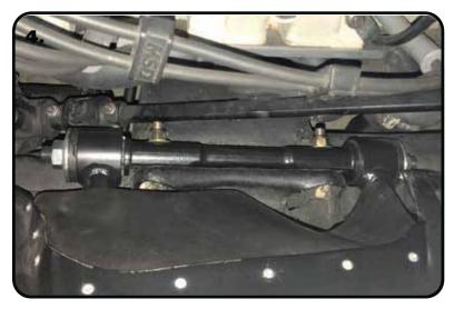
**4.** The Upper Control Arm is attaching the factory mount using factory hardware with the supplied 7/16" Flat Washer under the OEM Nut. Torque the nuts to 50 ft-lbs. The driver side arm is shown in **Figure "2"**. The Arrow on the Cross shaft points to the front of the car. **Page 4 & 5** has information about Caster and the Caster Slugs.
