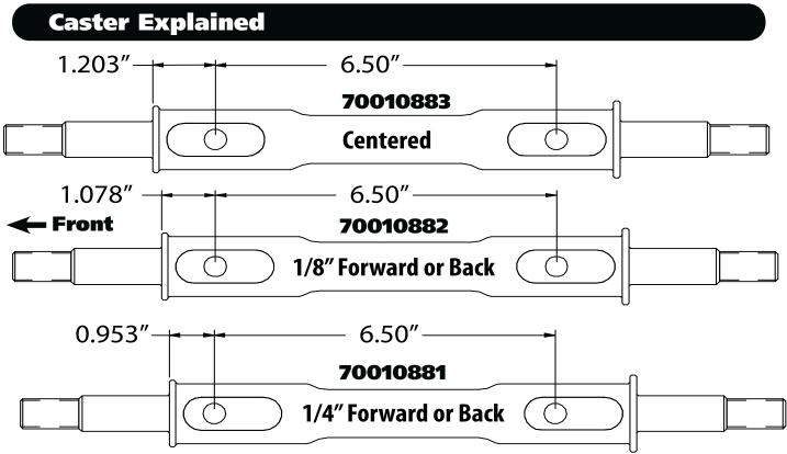
These StrongArms come equipped with a changeable caster slug setup. This allows you to add or remove caster from the front suspension, if desired. The caster slugs that come supplied in the kit are setup to be centered. The caster slugs allow you to add or remove caster without having to use a stack of shims. If more or less caster is desired, optional slugs can be purchased from Ridetech or your Ridetech dealer.
