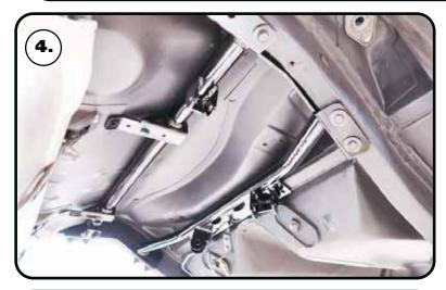
4. Steps 5-14 cover mounting the cradle into the car, review all steps. Image 4 shows the cradle installed in the car.
