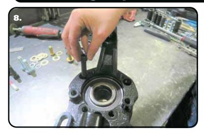
**8.** The Hub is attached to the spindle using (3) M12-1.75 x 40 SHCS. Apply RED Loctite to each of the mounting bolts. Insert them into the correct holes and Torque to 99 ftlbs.
