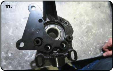
**11.** The caliper brackets are side specific. They have a D & P stamped in them. Lay the correct side caliper bracket on top of the shims, aligning the mounting holes with the mounting holes of the bracket. The counter sunk holes should facing up.
