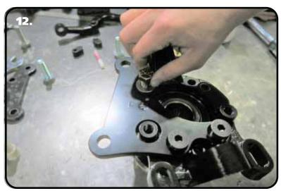
**12.** Insert a  $1/2"-13 \times 1 \ 1/4"$  flat head socket cap screw in each of the lower mounting holes. Install a 1/2" flat washer on a  $1/2"-13 \times 1 \ 1/4"$  hex bolt and insert it in the upper mounting hole. Tighten the hardware to 75 ft-lbs.
