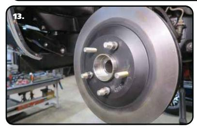
**13.** Install the rotor on the hub. Thread some lug nuts on the threads of the hub to hold the rotor tight on the hub.
