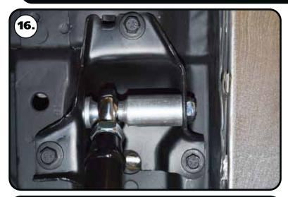
**16.** Attach the lower bar/mount assembly to the car. New 3/18"-16 u-nuts and 3/8-16" x 1 1/2" conical body Bolts are supplied in the kit. Install the u-nuts in place of the OEM u-nuts. Hold the assembly in place lining up the holes with the u-nuts. There is a tab bent up on the mount that indexes into a hole in the body. Make sure the tab is indexed into the alignment hole. Torque the mounting bolts to 30 ft-lbs.
