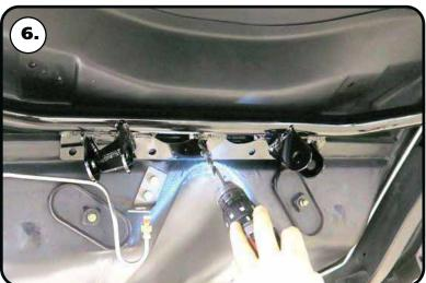
**6. Image 6** shows how the front tab overlaps the body seam. Multiple pieces of the car body overlap at this joint making it a strong area to attach to. Drill these 5 holes with a 3/8" drill bit using the cradle as a template.
