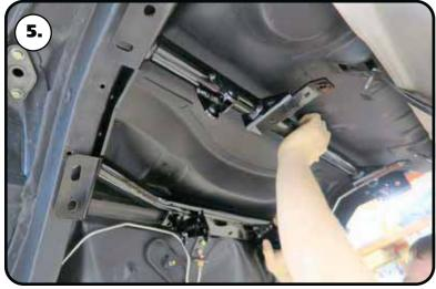
**5.** Install the cradle into the car. When the cradle is positioned properly, the front bar should be up against the body, the front tab will be up against the bottom side of the seam, and the sway bar mount tabs should be up against the bottom of the trunk pan.
