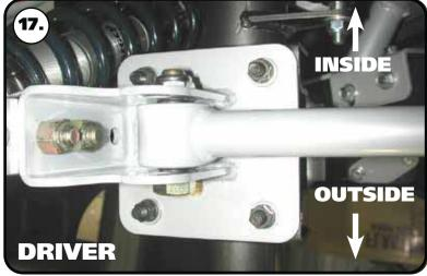
**17.** The lower axle bracket will be fastened to the leaf spring pad using the factory T-bolts/ U-bolts. The bar mount is offset to the inside of the car to provide more wheel and tire clearance. New 7/16" nyloks are supplied. Torque the nuts to 55 ftlbs.
