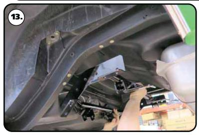
**13.** After you get all the riv-nuts installed, reinstall the cradle in the car. The bolts for the front tab and sway bar mounts can be reinstalled. Leave everything loose until all the bolts are started.
