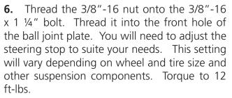
**NOTE:** If you are running the TruTurn setup, this steering stop bolt will not be used.
