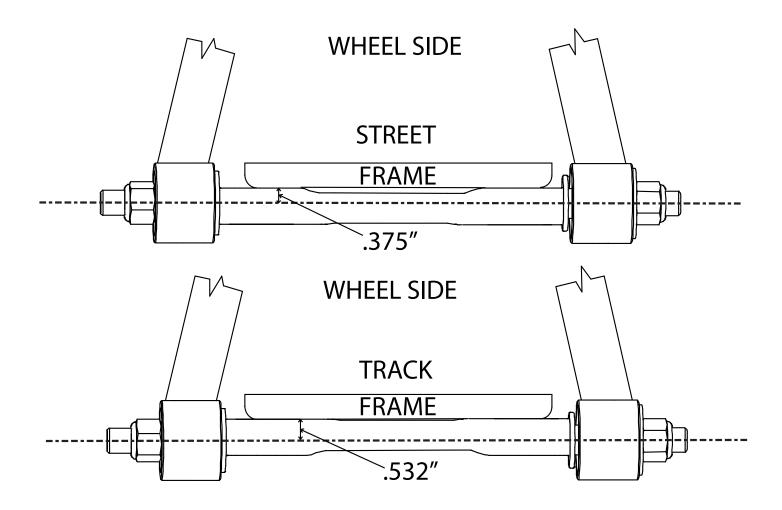
The cross shaft that is used in the upper control arms is offset. The offset combined with the caster slug option allows you to achieve the alignment setting you desire with minimal shims. To change the direction the Icon faces simply spin the cross shaft in the control arm.
