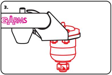
**3.** Install the ball joints in the control arms using **Figure "3"** as a reference. Torque the hardware to 9 ftlbs
