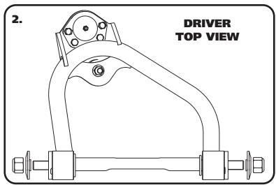
2. The upper control arm is attaching the factory mount using factory hardware. The driver side arm is shown in **Figure "2"**. The Ball Joint located on the arm to the rear of the car. Install the T-washers and 5/8"-18 lock nuts using **Figure "2"** as a reference. These can be tightened after installing the control arms on the car.
