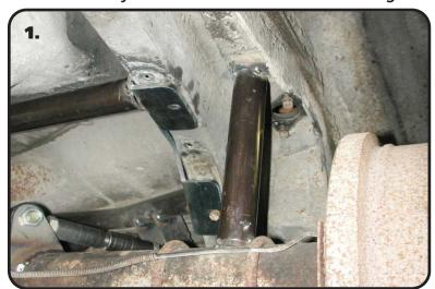
**1.** One helpful trick to help maintain ride height while setting up the rear MuscleBar is to put a spacer between the axle and the outside of the frame as shown in **Image 1**. This spacer should be 8 1/2" tall giving the Shock an eye-to-eye measurement of approximately 14 1/2".
