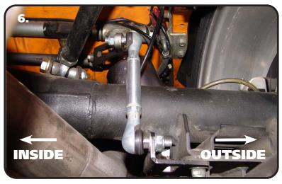
**6.** Install a 3/8" flat washer on the threads of one end of the PosiLinks. Insert the PosiLink into the hole of the musclebar arm with the threads pointing to the inside of the car. Refer to **Image 6**. Install a 2nd 3/8" flat washer on the inside of the arm followed by a M10-1.5 nylok nut. Repeat on the other arm with the threads pointing to the inside of the car. Torque the nuts to 37 ft-lbs.
