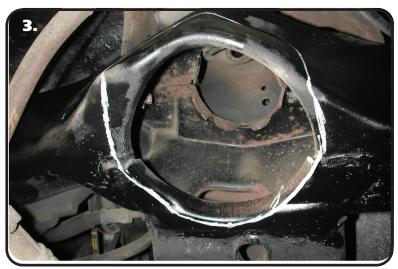
**3.** To allow clearance for the Shockwave, some trimming must be done on the inside of the coil spring pocket as shown by the white line in the picture. This is best done with either a cut off wheel or plasma cutter. Grind all cuts smooth when finished.
