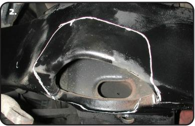
**2.** Some trimming must also be done on the outside of the frame pocket to allow clearance for the Shockwave.
