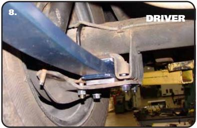
**7.** The top clamping plate with the large tab will sit on top of the leaf spring.
