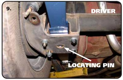
**9.** Install the lower clamping plate followed by the OEM lower mount **being sure the Pins and Holes are aligned**. Install the OEM hardware. Evenly tighten the hardware in a crisscross fashion. Torque the nuts to 55 ftlbs.
