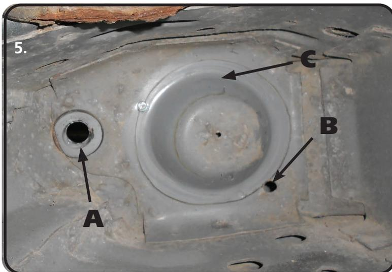
5. Picture "5" shows the factory upper coil spring pocket in the car. (A) is the factory shock hole that the upper plate and mounting bracket will be bolted through, (B) is a locating hole in the body that will be used to help locate the new upper plate, (C) is the factory coil spring locator that will also help in locating the upper plate
