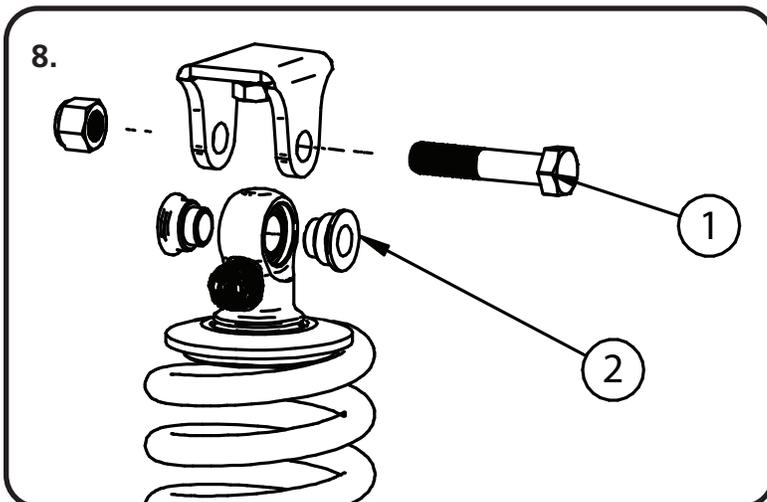
**8.** Install the 1/2" I.D. Spacers (1) into the bearing of the upper CoilOver eyelet. Insert the CoilOver into the upper mounting bracket aligning the holes in the spacers with the holes in the bracket. Insert 1/2" x 2 1/2" bolt through the bracket and CoilOver. Install 1/2" Nylok nut and tighten.
