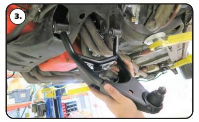
**3.** Insert the control arms into the OEM mounts.
