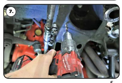
**7.** Use a 3/8" drill bit to drill a hole at the center of the bump stop spacer.
