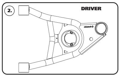
**2.** After removing the factory lower control arm, clean the bushing mounting surfaces on the frame. The control arms are marked "D" for Driver and "P" for Passenger. The ball joint pin points up and the sway bar mount is on the front side of the arm. **Image 2** shows a top view of the driver side control arm.
