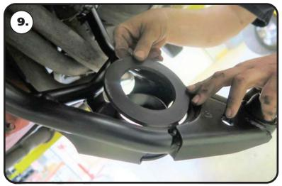
**9.** Use the guide on **Page 3** to determine what shims, if any, to use to achieve the desired ride height. Place the shims over the center ring. They will sit flat against the floor of the control arm.
