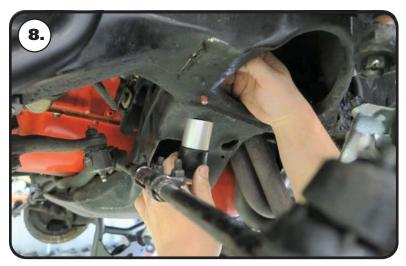
**8.** Install a 3/8" split lock washer & 3/8" flat washer on a 3/8"-16 x 3/4" bolt. Apply red loctite to the threads of the bolt. Insert the bolt in the drilled hole by reaching into the coil spring hole. Align the bump stop spacer with the bolt and thread it into the spacer. Tighten the bolt to 12 ft-lbs.
