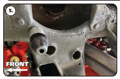
**5.** The kit includes new bump stops. **Steps 5-8** will help guide you in the installation of the bumpstops. The bump stop will be installed at the front inner edge of the coil spring opening. **Image 5** shows the bump stop installed as a reference. A hole will need to be drilled to attach the bump stop to the frame.
