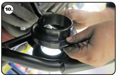
**10.** Place the coil spring isolator over the ring of the control arm.
