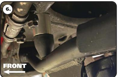
**6.** Thread the bump stop into the aluminum spacer. Swing the control arm up to help determine the proper location of the bump stop. The bump stop needs to contact the front tube of the control arm with the aluminum spacer sitting flat against the frame. Mark the outside edges of the spacer as you will need to drill a 3/8" hole at the center of the location.
