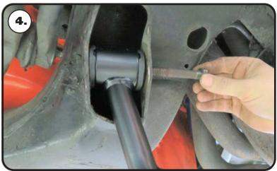
**4.** Line up the OEM mounting holes with the through holes of the bushing sleeves. Install a 1/2" flat washer on each of (2) 1/2"-13 x 3 1/2" bolts. Insert the bolt/washers through the mounting holes. Install a 1/2" flat washer and 1/2"-13 nylok nut. Torque to 75 ft-lbs.
