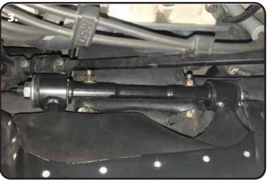
**3.** The Upper Control Arm is attaching the factory mount using factory hardware with the supplied 7/16" Flat Washer under the OEM Nut. Torque the nuts to 50 ft-lbs. The driver side arm is shown in **Figure "2"**. The Arrow on the Cross shaft points to the front of the car. Page 4 & 5 has information about Caster and the Caster Slugs.
