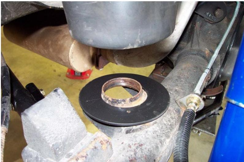
6. Place the large lower air spring plate over the lower coil spring retainer.
