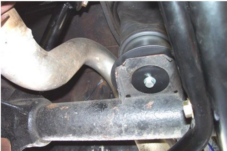
9. Secure the air spring to the axle using a 3/8" x 1" bolt, lock washer, flat washer, and the 2 1/2" washer.
